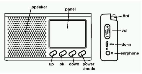
DC-in: 5V dc-in battery charge
